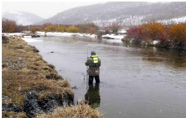
A Hydrologic Technician manually measures streamflow at USGS streamgaging station 13063000 in Idaho. Credit Marshall Williams USGS
